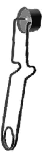
Used to light Bunsen burners – squeezing the handle drags a flint across a steel rasp inside the cup. This produces a spark
