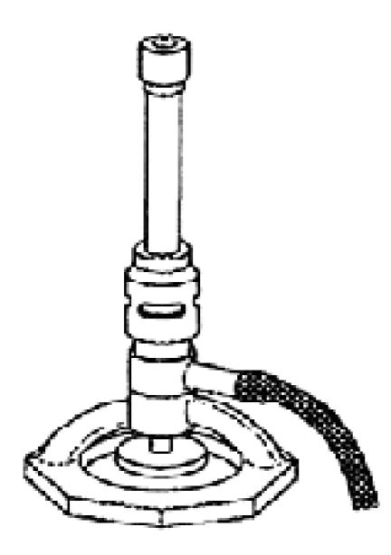
Attached to a gas outlet, and used to heat substances and to do flame tests.
