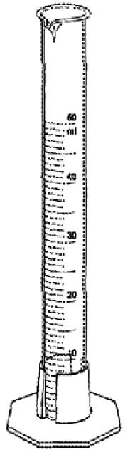
.THE ONLY piece of glassware that can be used to ACCURATELY measure a liquid.
