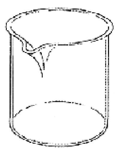
•Used to contain a liquid while mixing, heating, cooling, etc.
