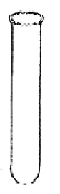
•Used for holding small amounts of a substance while mixing, heating, cooling, etc.
